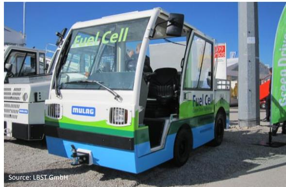
The overall aim of the HyLIFT projects is to conduct large scale demonstration of hydrogen fuel cell materials handling vehicles to accelerate commercial market introduction of this technology.
